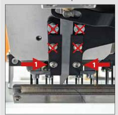
Now please loosen and remove ONLY the lower screws [1] on the plate. Do not loosen any other screws here.
