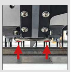
Carefully loosen and remove the screws. The protective bracket can now be easily removed.
