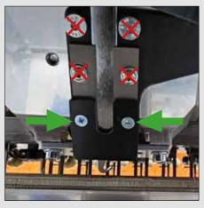
Now align the new guard as shown in the picture above. Secure it with the screws provided. Use the screw threads of the screws you removed earlier.
